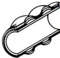
Fig I-4. Air Trapped in Rewound Roll
