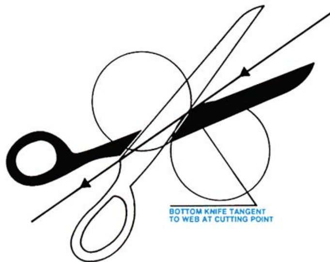
Fig II-4. Shear Slitting Principle
