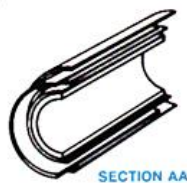
Fig I-2 and I-3. Air wound between layers showing the relative shifting of the material.
